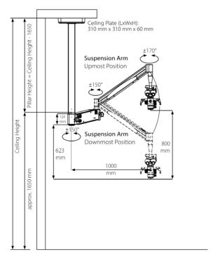
Maintains ground clearance. Pillar height can be adjusted to any ceiling height.
