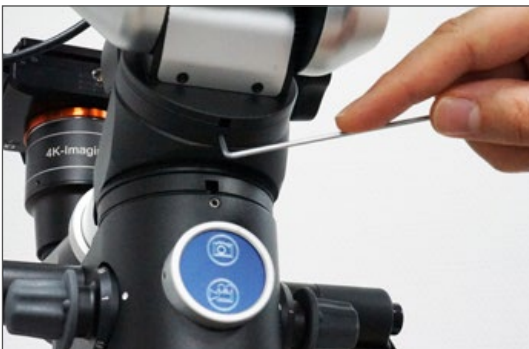
3. Assemble binocular and tiltable tube to ergo optic (2 mm Allen wrench).
