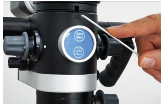
2. Assemble lighting unit to ergo optic. (2 mm Allen wrench).
