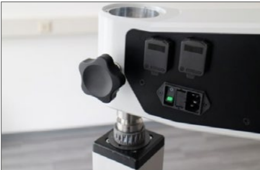
5. Attach suspension arm to guide bearing.
