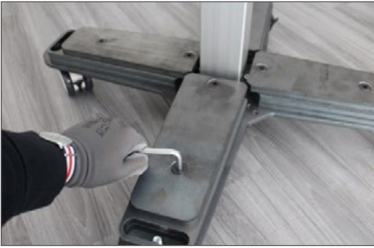
7. Assemble balance weights. Note that the counter screws are put back in place (wrench size 19 mm).
