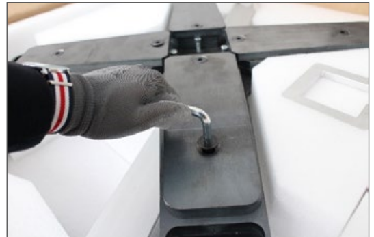
2. Remove the balance weights by loosening the screws with an 8 mm Allen key. The screws are secured at the bottom with M12 nuts (wrench size 19 mm).
