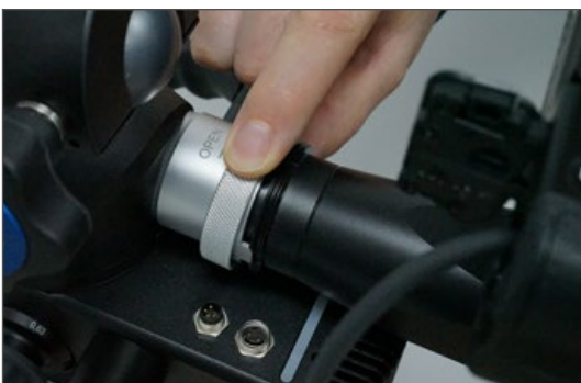
5. Fit adapter in optical connector and save with ring.
