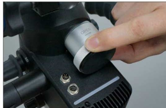
4. Remove dust guard from optical connector.
