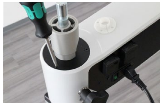
6. Assemble mount (take care of angle position).
